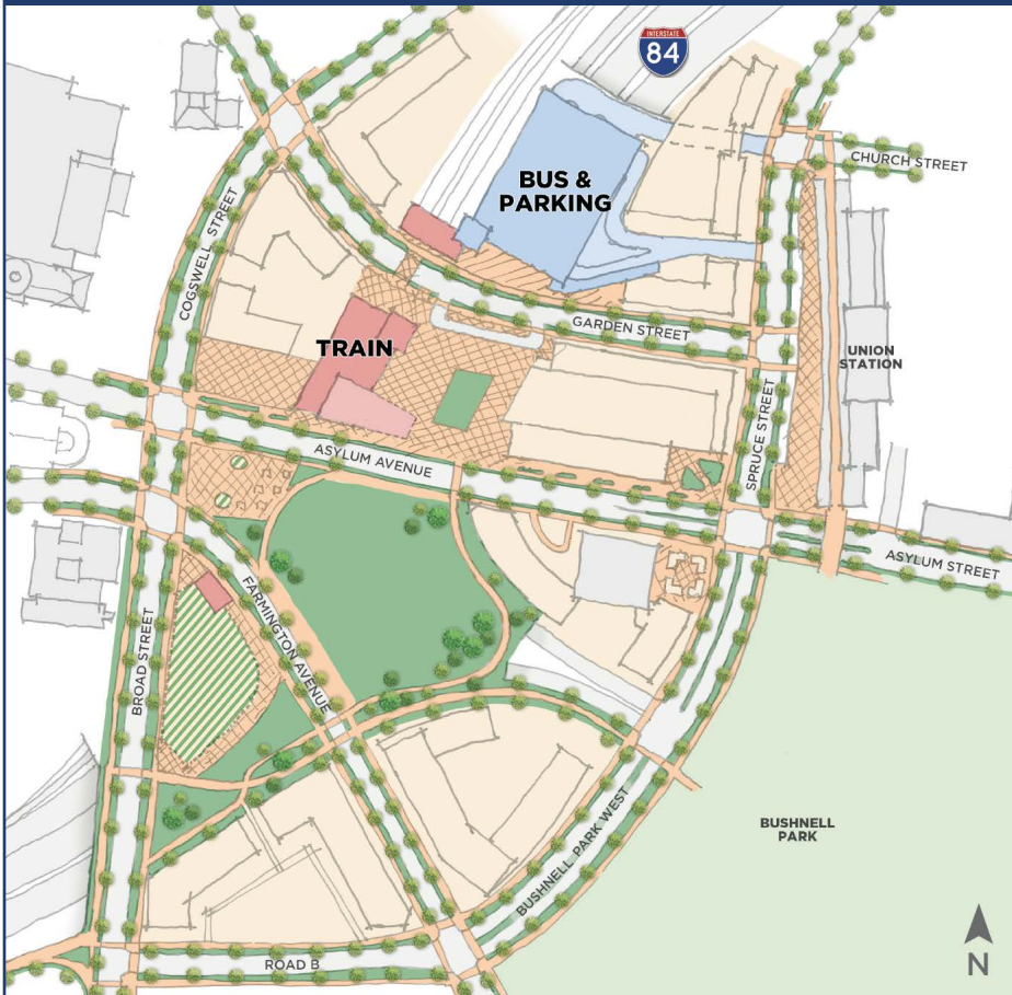
Northern Concept E1, so named due to its position north of Asylum Avenue, sites the multi-modal station as well as the bus and parking facilities, on capping north of an extended Garden Street.
